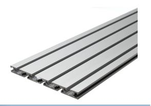
Solid profile from anodized aluminum, intended to be used as a base plate, eg. in a CNC machine or similar. The large thickness prevents it from bending under stress.
