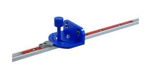
Slider with adjustable angle, intended to be used with the fence profile. Can be used for an adjustable sled for a table saw and similar. The angle is easily readable and can be locked using the knurled knob.
