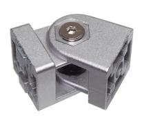
Tiltable arm for series 30 profiles. The arms an be mounted on the side or at the end of the profiles. There are locking taps included, that fit in to the ends of the arms, så that they are locking in to the tracks of the profile, or in the ends
