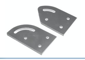
Smart brackets made of solid 6mm aluminium, that are rotatable 45 or 90 degrees. They can be used for fixed, adjustable, and movable joints, depending on the accessories you use. The holes and slots are for 8mm bolts. Locking handles are an obvious choice in the slot if you want an adjustable joint.
