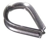
Thimble that is used for protecting a wire-loop against wear. It is inserted into the joint, and prevents the part put through the loop from wearing the strands.
