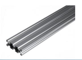
Tripple v-slot profile in extruded and annodized aluminium, with a total of 8 smooth tracks for v-slot wheels. The profile is available in 1, 2 and 3 meter lengths.
