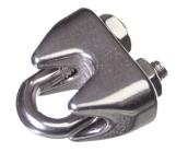
Solid clamp for locking one or two wires together. The clamp is locked by fastening the two nuts. The clamp is made from stainless steel A4.
