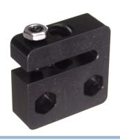
Block with transverse lead screw thread, with built in anti backlash. The pinol screw is tightened until the backlash is gone.
