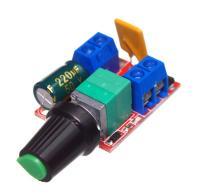
Extra compact PWM regulator for controlling the speed of a DC motor, with speed from 1% to 10%. Note that the motor will drop its performance as you lower the speed. This regulator will perform much better compared to just dropping the voltage.
