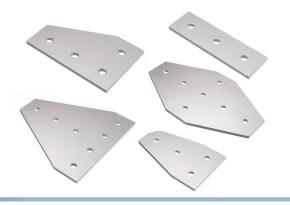
Extra strong bracket milled out of 4mm aluminium, that is annodised afterwards. The holes fit M6 bolts. The different models can be used for various types of joints.
