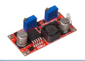
Compact regulator that can step down the voltage from 35V down to 1.5V, and limit the current from 2A and down.
