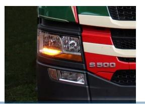
Complete set LED emitters that replace the original xenon white with eg. yellow. Fits Scania +2016 trucks, with halogen headlights.
