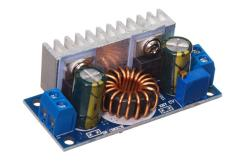
Compact step up DC boost converter with max 8A input current. The voltage can be boosted up to 42V, adjusted with the small potentiometer. Max current on the input is 8A, and 5A on the output.
