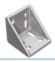
Large angle-bracket in cast aluminium for 6060 profiles in series 30, with two by two M8 mounting holes. The thickness of the bracket is 5mm.
