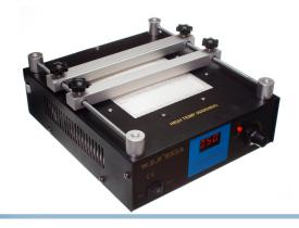
Preheater that is used for soldering or repairing circuit boards. It preheats the board so that components can be soldered or replaced easier. Typically you heat the board to +100 degree, where after you use a SMD hot air soldering station, or a soldering iron, to raise the temperature on the individual components, that need to be soldered or replaced.
