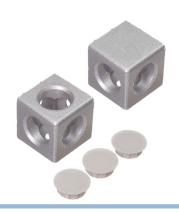
Smart corner join that is used for screwing two or three profiles together in a corner, eg. in a box. You simply cut threads in the end of three profiles, where after you use a button head bolt for fastening. Notches on the join that go in to the profile ensures that the profiles cannot be twised loose. This gives you a secure, solid and stiff joint.
