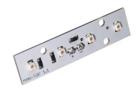
LED emitters 24V that replace the original circuits in the top lights on the new MAN trucks. The original emitters are taken apart by removing two metal clips, where after the board is taken out and the new put in.
