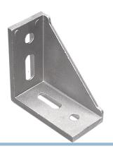
Extra large angle bracket, that gives extra stiffness and strength in the connection, compared to standard. There is space for 4 pcs M6 bolts in the bracket. You should use 14 or 16mm bolts together with a washer.
