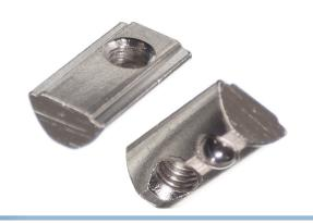
T-nut that fits in to series 30 profiles. Can be pushed in to the slots anywhere. The spring in the bottom locks the nut.
