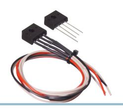
Simple rectifier bridge, that ensures that you always get the correct polarity connected. The voltage from outside is connected to the input pins, where after the voltage on the output pins will be correctly polarized on the plus and minus pins.
