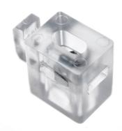
Block that is inserted in to series 30 profiles. The M6 bolt in the block can be used for tightening plates between profiles.
