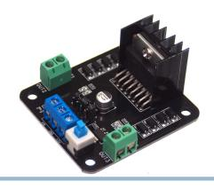
Simple and effective motor controller for 1 or 2 DC motors, with a voltage up to 24V, and max current of 2A. each channel. (Total 4A)
