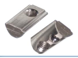
T-nut that can be pushed in to the tracks on series 40 profiles. The spring avoids it gliding and falling out again.
