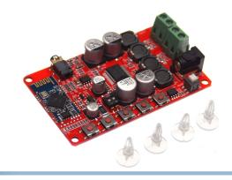
Amplifier module with built-in Bluetooth and analogue input (3.5mm plug). The module can play music and other sound wireless over Bluetooth 4.0 from smartphone, tablet and PC. The amplifier has 2 outputs of 50W outputs.
