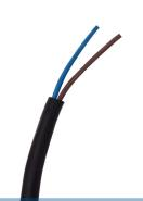
Flexible cable intended for mounting in dry, humid and wet environments, on machines, tools, lamps, motors etc. Maximal voltage is 750V phase to phase, 450V phase to ground and 1000V on fixed protected installations.
