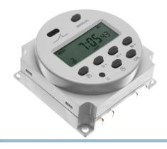
Smart and compact timer relay that is controlled by time and weekday, as well as workday/weekend and other patterns. The relay must be supplied with 12V, but the internal relay can switch 230V, up to 10A. The built-in backup battery, lets the watch tick without supply, with a life span of up to 3 years.
