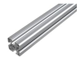
Standard construction profiles in 4040, with basis dimensions  $40 \times 40 \text{mm}$  and a 8mm slot. The profiles are an extra thick model, solid core and round holes.
