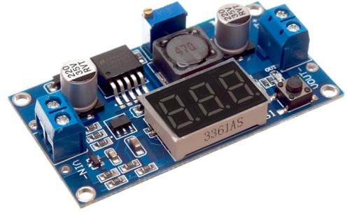
Compact voltage regulator with built-in display, that can show output and input voltage. The output voltage is easily adjusted with with screwdriver on the small potentiometer. Counterclock wise reduces the voltage, clockwise increases it.
