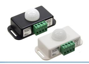
Compact PIR motion sensor with screwterminals on the input and output. The sensor can be used for both 12V and 24V. When the sensor is activated, it will turn off after the set up delay, that can be from 1 to 10 minutes.
