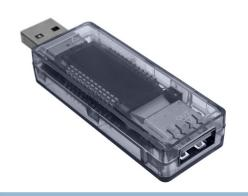
USB charging-tester, that measures and displays charged capacity, charging voltage and current in the large display.
