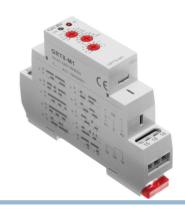
A compact timer with 10 different functions that can be used for timecontrol and automatics. The time interval can be set from 0.1 seconds up to 10 days. Mulitple controllers and relays can be connected for making advanced automated controls.
