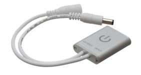
A dimmer that is mounted on the backside of wood or glass-sheets, where it can register touch through the material. It can be mounted on surfaces with up to 30mm thickness, for example tables, doors, etc. This makes it possible to do a completely invisible installation.
