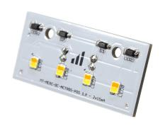
A special lightsource that replaces the original white LED light sources in Mercedes Actros' top position lights. The pins and LEDs are as standard, so replacing these is simple with the correct tool.
