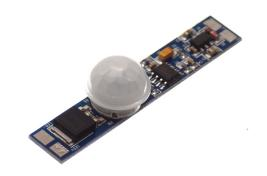
Motion sensor that is incredibly small. It can be used for eg. LED strips, and it is perfect for mounting in a LED aluminum profile. The sensor turns itself off after it has not registered any movement in 1 or 5 minutes, depending on the chosen model.
