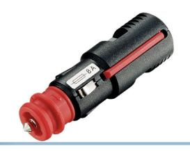
A cigar-plug that is easy to connect with the built-in screw terminals. It is available with or without a built-in 8A fuse, which ensures that you avoid problems if shortscircuits happens.
