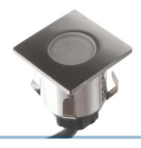
A square LED spot, 35x35mm in stainless steel. Can be used outdoors on balconies and on ceilings. It gives a warm white light. The spot has a holediameter of 32mm.
