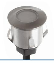
A round 35mm LED spot in stainless steel. Can be used on balconies or ceilings, creating a nice atmosphere. The spot has a hole-diameter of 32mm and a mounting depth of 36mm.
