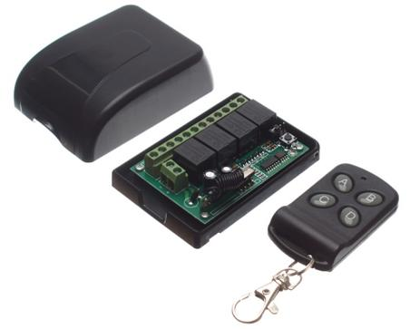
A relay-controller for 12V or 24V with 4 channels, which are set by a wireless remote, 433mhz. The 3 built-in functions give you many possibilities.
