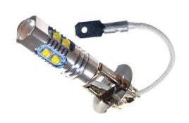
A very bright H3 LED bulb that fits in to the original sockets. With  $10 \times 5W$  CREE LEDs, it is equivalent to a 40W incandescent bulb. This means that they are not bright enough to replace the original H3 bulbs on 55W, so you can only use them for DRL. The light-color is xenon-white (6000K) or yellow/orange.
