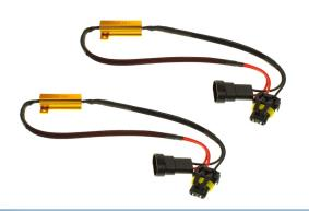
A resistor with a 9005 plug. Used for LED conversions, where it is put in between the 9005 bulb and the car' 9005 plug.
