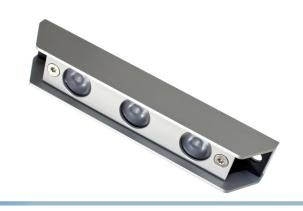
Our LED lamps for underwater light have 3 powerful High Power LEDs in one single color. The solid aluminum and plastic surface make the lamp water impact resistant, while potting the Electronics in polyurethane makes the lamp completely waterproof. This combination creates a lamp that is perfect for mounting under water.
