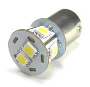
BA15s LED bulb with 7 pcs. 5050 SMD diodes that make a wide illumination. The bulb may replace a regular 5  $\sim$  10 watt incandescent bulb in the parking lights and in the tail lights.
