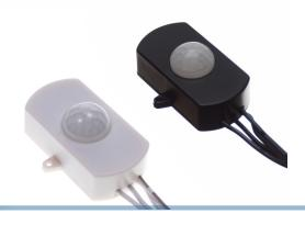
A smart little motion-sensor and a light sensor with a DC plug at the entrance and at the end, so it can be connected to our power supplies. As soon as the sensor sees movement, it will open up the power at the end, with the same voltage as the input. 12V, 12V out. If you want to use DC connectors with screw terminals, you need to use DC connectors with a 2.1mm inner diameter.
