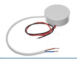
LED driver that delivers 700mA constant current. Max voltage 12V, and can pull up to 3  $\times$  3W High Power LEDs.
