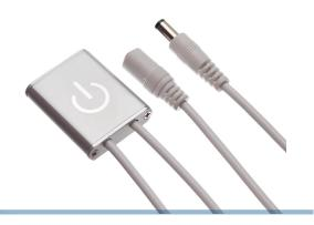
This smart touch dimmer can be used for both 12V and 24V products. The dimmer is very compact and it is controlled via a touch on the surface. There is an easy on/off power options and it can remember the last brightness set. It is available with a 2-metres wire or DC plugs on 30cm cables.
