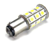
An extra heavy BAZ15D Xenon White LED bulb with 24 pcs. 5050 SMD diodes, which together make 270 lumens. The LED bulbs are used for the run/position lights. The LEDs bulb location makes the whole dish to light up. The bulb has a built-in voltage regulator that protects from overvoltage and thereby also provides a longer life.
