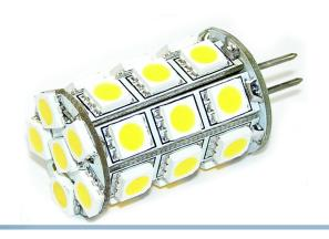
G4 LED bulb with 27 pieces SMD diodes, which together produce a 370 lumens warm-white light. The brightness is equivalent to approximately  $\sim$  40 Watts.
