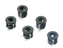
Plastic mounting frames for 3 mm indoor diodes. The framework enables an easy mounting of the plastic shield on scooters or others. They must be inserted in a 4.5-5.0 mm hole.
