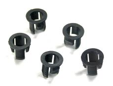
They are suitable for outdoor and indoor 5 mm LEDs and 3 mm diodes. The framework enables an easy mounting of the plastic shield on scooters or others. They must be inserted in a 6.5 mm hole.
