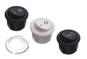
Switch with various functions, in black or in white plastic. It can be used for 12V, 24V and 230V. Panel-mounted in a 21mm hole. The panel-thickness can only be 0.7-3mm.
